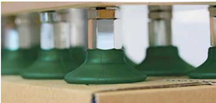
Suction gripper matrix with rigid fittings for handling cardboard boxes
