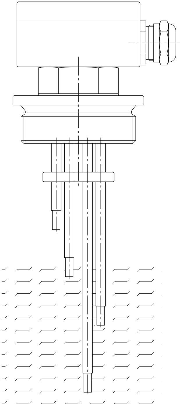
Electrodes are electrically conducting rods that can be used to monitor and control filling levels. They work on the principle of conduction in association with level controllers (see chapter 1011). If the electrodes are immersed in an electrically conducting liquid, the resulting current activates high-voltage, potential-free, relay contacts via a signal amplifier.
