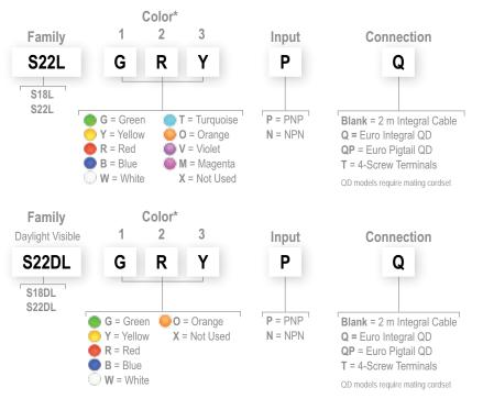
\* Single-color models are available and should be ordered as PNP, but can be wired for either PNP or NPN input
