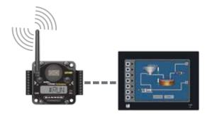
Central monitoring of machine status with Banner's Wireless products allows users to easily analyze productivity and efficiency. Banner's Wireless Gateway can connect directly to an HMI or other control system to send status messages via email or text.
